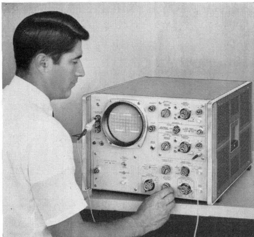
Fig. 1. -hp- Model 175A Oscilloscope uses new high-sensitivity -hp- cathode-ray tube to obtain dc-50 megacycle performance with simplified circuitry. New crt is also free of deflection defocusing so no astigmatism control is needed.
